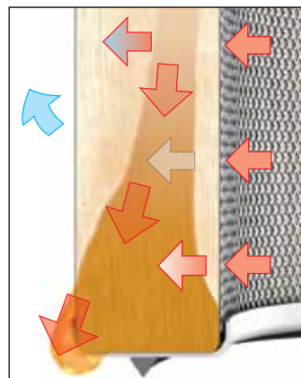
The diagram shows the downward flow of the droplets. The combination of flow and hydrodynamics forces the sedimentation out.
