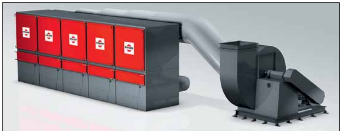
Central separator consisting of five AERO® modules of size 3 and one fan (nominal air flow of 64 000 m 3 /h)
