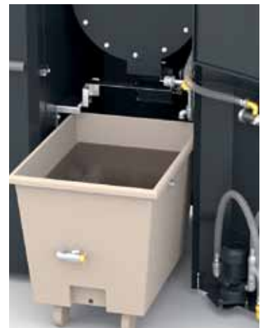
Easy discharge of contaminated process water
