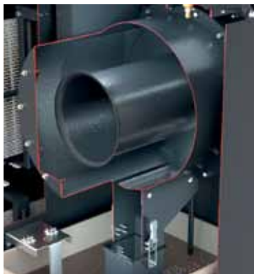
Cross sectional view: Demister and immersion nozzle for discharging process water into the process water tank.
