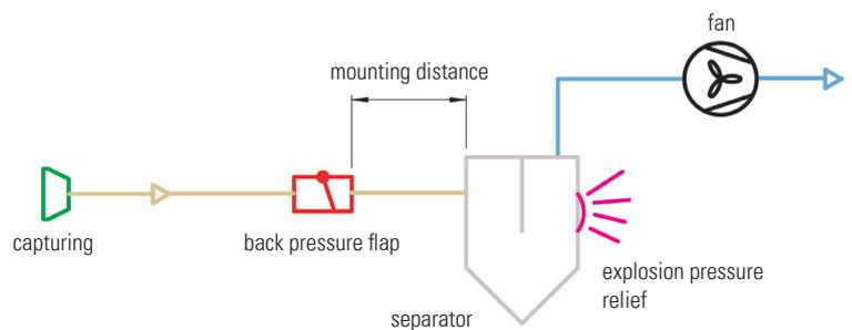
Staff working at the collection points or system components at the suction side are protected against the impact of explosions.
