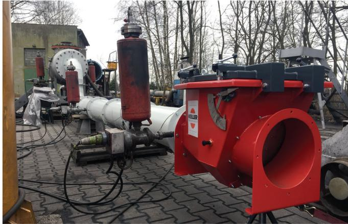
Back pressure flaps must comply with the stricter test standard (EN 16447).
