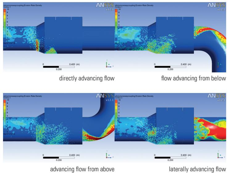
**CFD ProFlapIII NS315 simulation parameters:**
