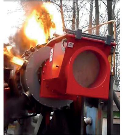
ProFlapIII with explosion protection module B
